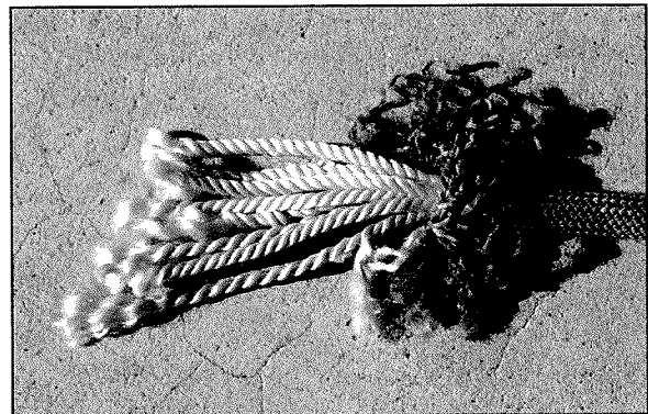
Figure 2-2: Dynamic Rope Core and Sheath
