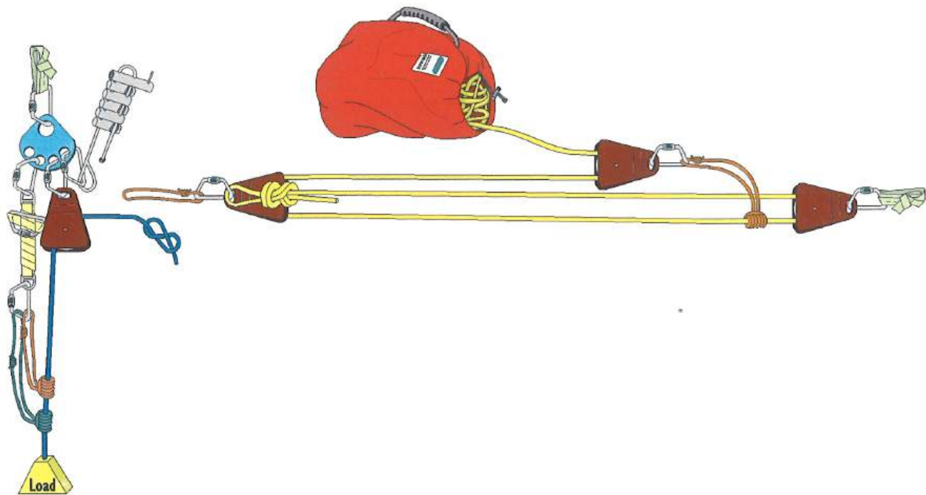
Figure 11-28: Construct 5:1 Pig Rig
