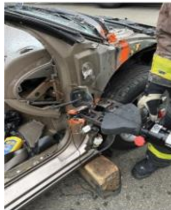
Cut Lower A-Post Just Above Hinge
