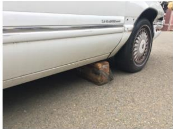
Proper Placement of a Step Chock
