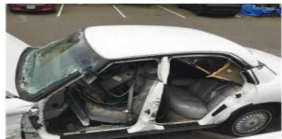
Figure 6.4: Hinging the Roof
