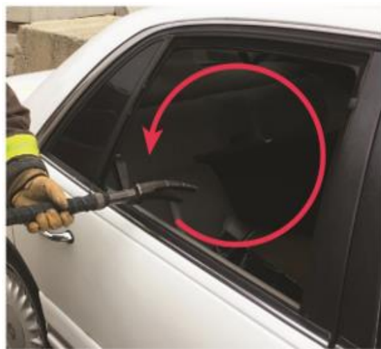
Sweeping with a Tool to Clear Glass
