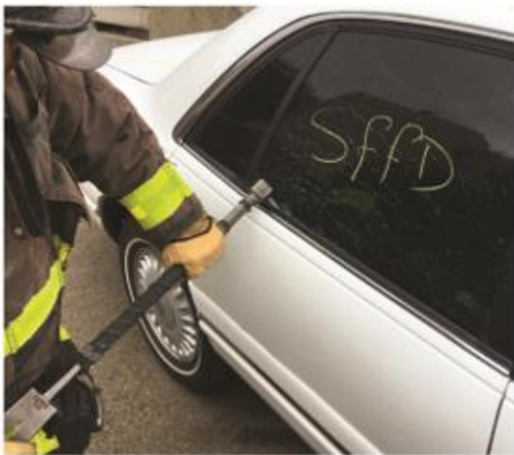
Breaking a Rolled-Up Window with a Halligan (Pry Down)
