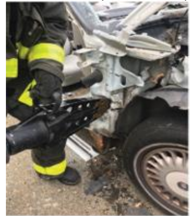
Place Spreader Tips In Lower A-Post "Notch"
