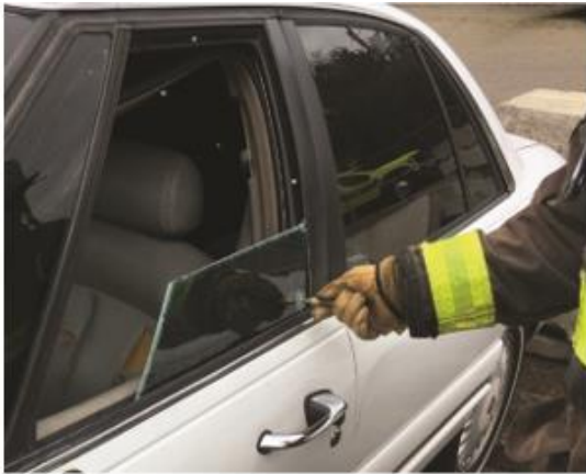
Breaking a Rolled-Down Window With Center Punch
