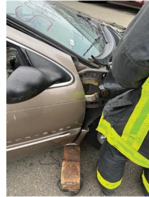
Spread the Hinge to Fail or Cut the Hinge (Not the Pin)
