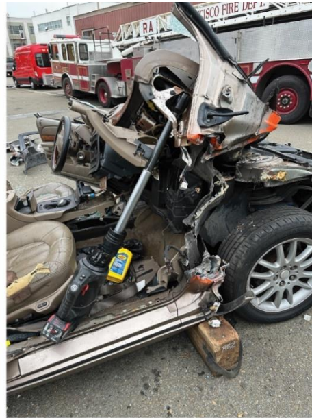
Ram Extended in a Dash Roll
