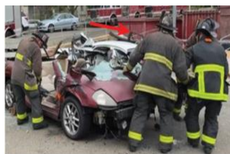
Pull Roof to Shear Windshield
