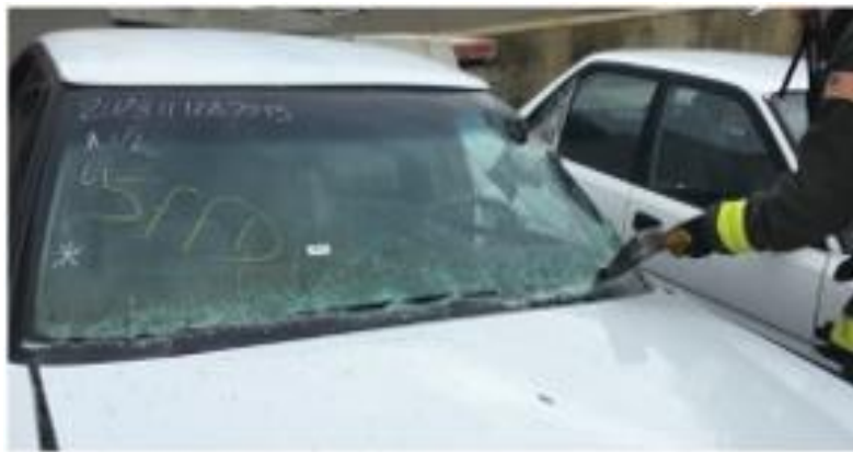
Cutting the Bottom of the Windshield
