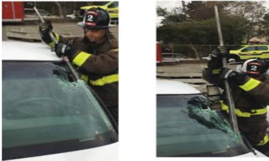
Breaking a Windshield Along the A Post with a Prybar
