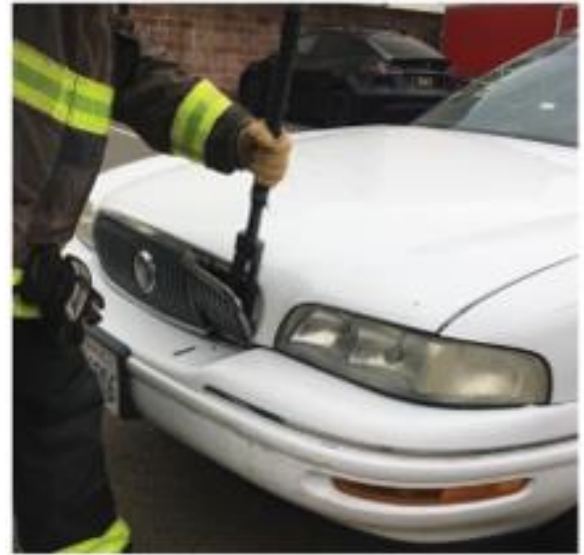
Removal of Front Grill
