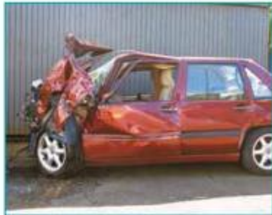
deformation due to crumple zones
