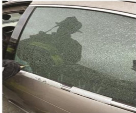
Breaking a Rolled-Up Window with Center Punch
