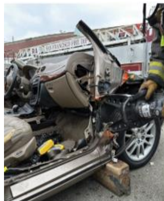
Dash Lift and Step Chock
