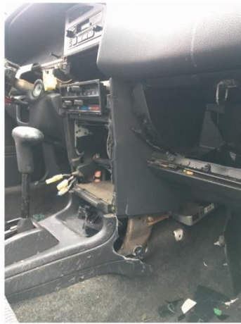
Pull Plastic at Center Console
