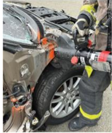
Cut Upper Subframe Relief Cut (OPTIONAL)
