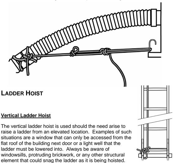
To better facilitate the raising of the ladder on a roof or the placing of a ladder in a light well, the ladder should be tied so that the butt of the ladder is raised first. The vertical ladder hoist is tied using a bowline knot.
