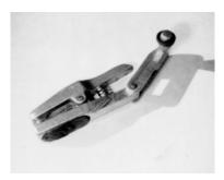
The **Quick Fit Sprinkler Shutoff** is used to shut off water flow to all types of sprinkler heads. Results may not be as good when using on a recessed head. The jaws end is inserted into the sprinkler head and the fulcrum lever pulled down thereby opening the jaws and causing the tool to open and place pressure against the water flow from the sprinkler and therefore shutting down water flow.
