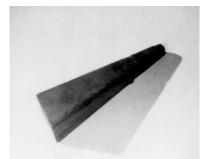
The **Redwood plug** is a quick and efficient manner of closing down water flowing from a sprinkler head. It is tapered and made of soft redwood which allows the tool to be inserted into the fused sprinkler head. Tap lightly with a axe to seat the tool and water flow will be stopped. Do not confuse the redwood sprinkler head with the redwood plug for broken pipes. The sprinkler tool is square at the large end and tapered; the
