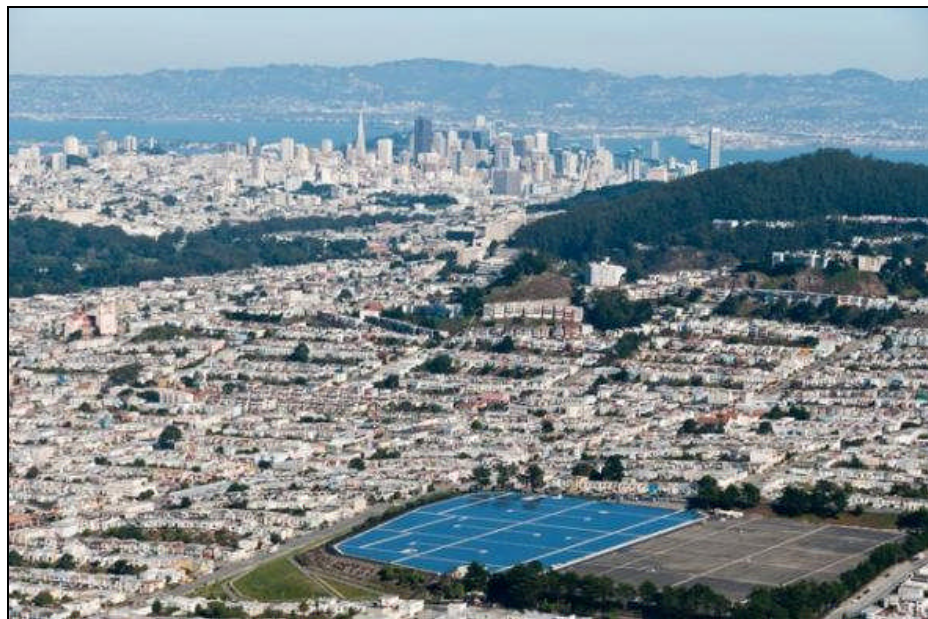
Figure 38 – 5 megawatt Sunset Reservoir PV system.
