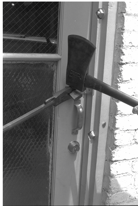
With the shackle between the fork, a striking surface is provided for the ax.
