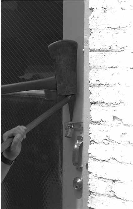
Using the point of the Halligan tool to drive the hasp and lock off the door.
